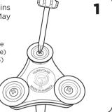
Carefully place new rubber foot onto pivoting head foot cavity.
